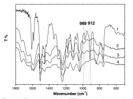
Figure 1 Comparison of the FTIR spectra of epoxy phenolic resin (1), modified epoxy phenolic resin (2) and modified epoxy phenolic resin treated at 120  $^{\circ}$ C (3) and 140  $^{\circ}$ C (4)
