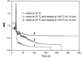
Figure 2 Comparison of the dissolving rate of the resin films (film thickness: 20-25 nm)
